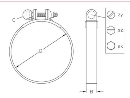
C (screw type) = SZ Diameter D = 114 Width B = 20
